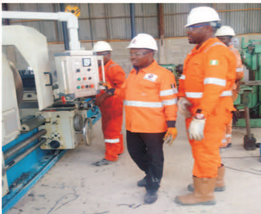
TEST-RUNNING OF NEWLY INSTALLED SEMI AUTOMATIC OIL COUNTRY LATHE BY EVERPRAISE ENGINEERS AND TECHNICIANS
