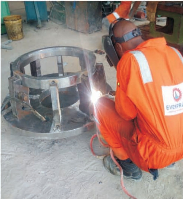
FABRICATION OF SPLIT-TYPE BASE PLATE LANDING RING
