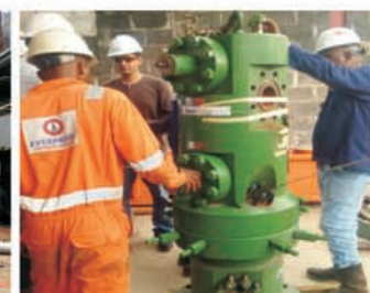
SUCCESSFUL SIT ON MODIFIED XMAS TREE & TUBING SPOOL AT EVERPRAISE FACILITY
