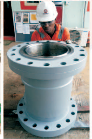
MANUFACTURED RISER SPOOL (135g" - 5K TOP & BOTTOM)
