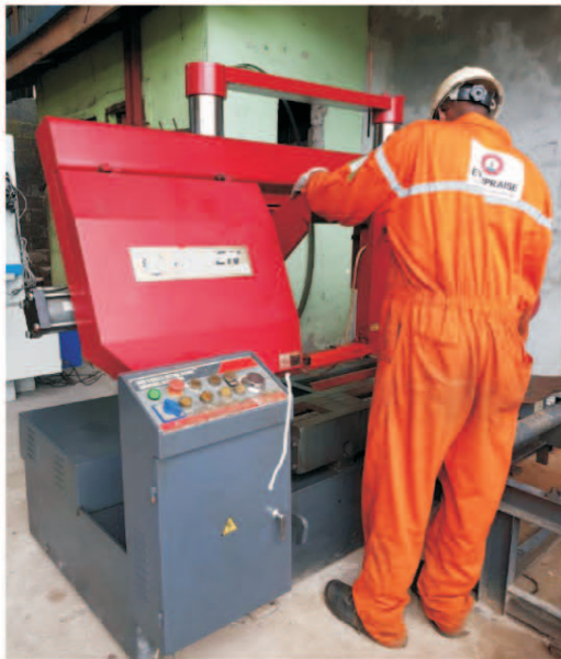
BAND SAW WITH 500MM CUTTING CAPACITY
