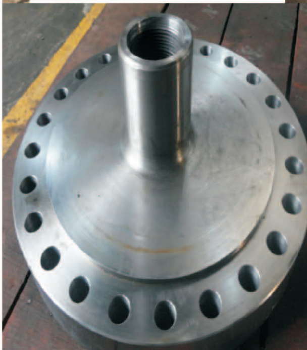
MANUFACTURING OF 13-5/8" 5K FLANGE X 4 1/2 " IF BOX CONNECTION
