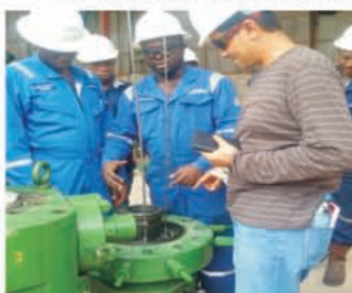
DUMMY TEST CARRIED OUT BY SCHLUMBERGER ENGINEERS ON XMAS TREE AND TUBING SPOOL MODIFICATION
