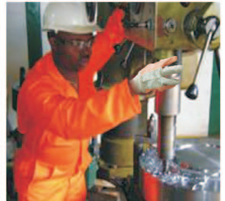
DRILLING OF BLIND FLANGE ON RADIAL DRILLING MACHINE
