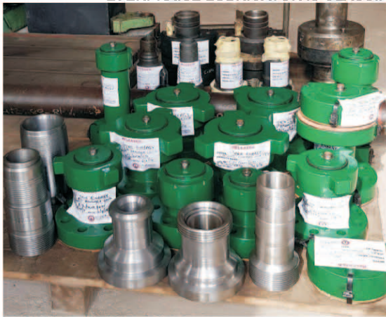
MANUFACTURED HUB WITH WECO CONNECTIONS, ACME CROSS OVERS AND TREE TOP CONNECTION WITH HAMMER UNIONS
