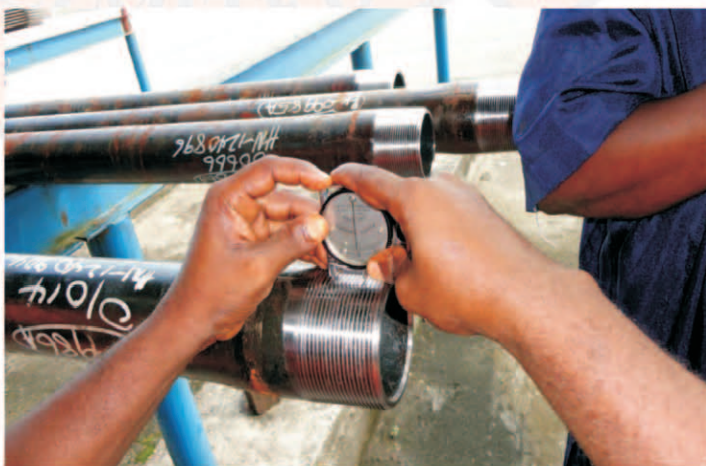
LEAD MEASUREMENT ON A TUBULAR JOINT
