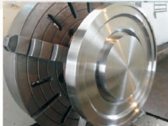
EVERPRAISE TECHNOLOGIES, MACHINES OF FLANGE FOR SUBSEA XMAS TREE
