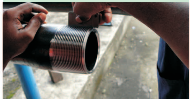
CHECKING THREAD PROFILE ON A TUBULAR JOINT
