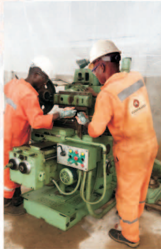
SLOTING OF INTERNAL SPLINES BY EVERPRAISE MACHINISTS ON A UNIVERSAL MILLING MACHINE
