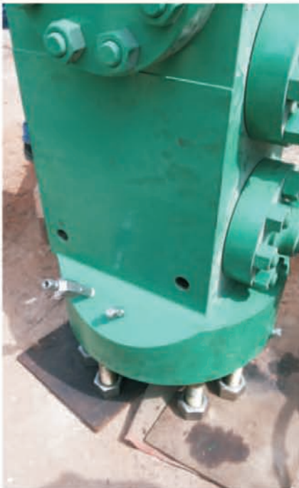
NEW ESP PORT CREATED ON CAMERON XMAS TREE BY EVERPRAISE
