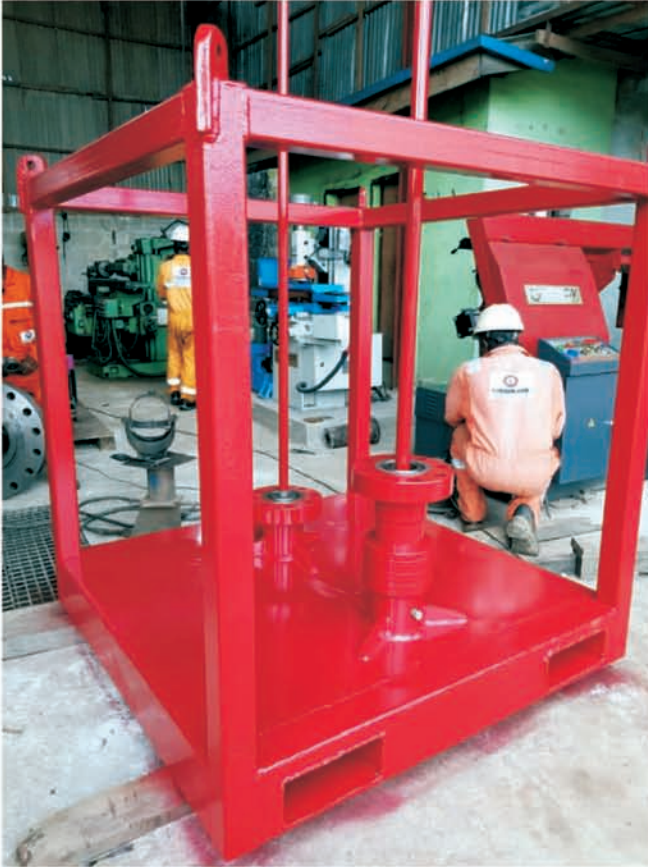
FABRICATION OF BOP TEST STUMP WITH PULL BAR
